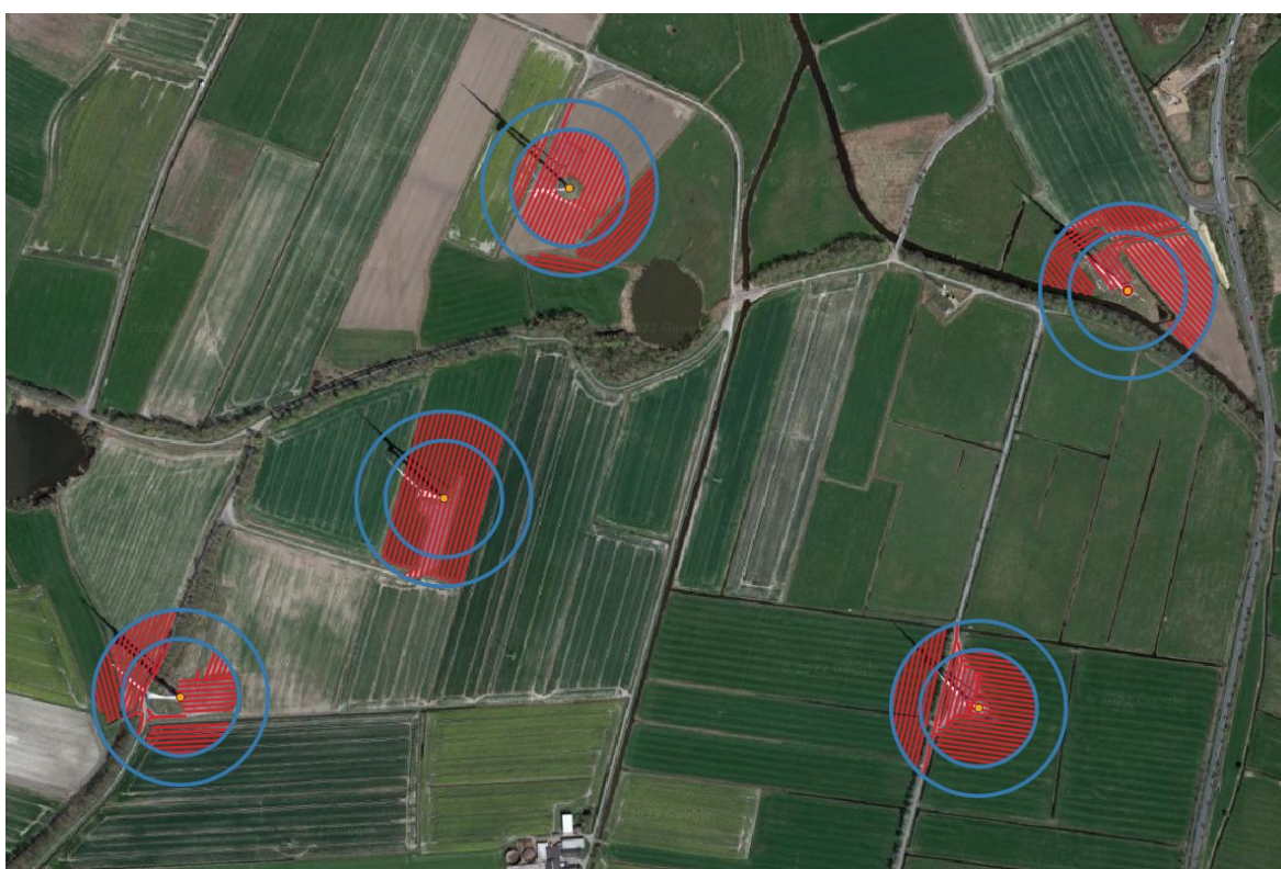
Figure 3-10 Overview of test area with all five turbines indicated with orange dots. Red lines show transect design for carcass searches. Inner blue circle indicates 80 m and outer circle indicated 120 m radius around the turbine.
